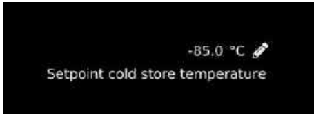
Fig. 60: Cooling chamber temperature set point icon
