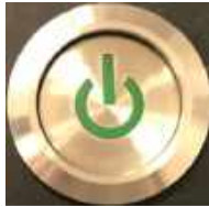
Fig. 29: Main battery switch pressed
