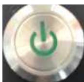
Fig. 32: Main battery switch
